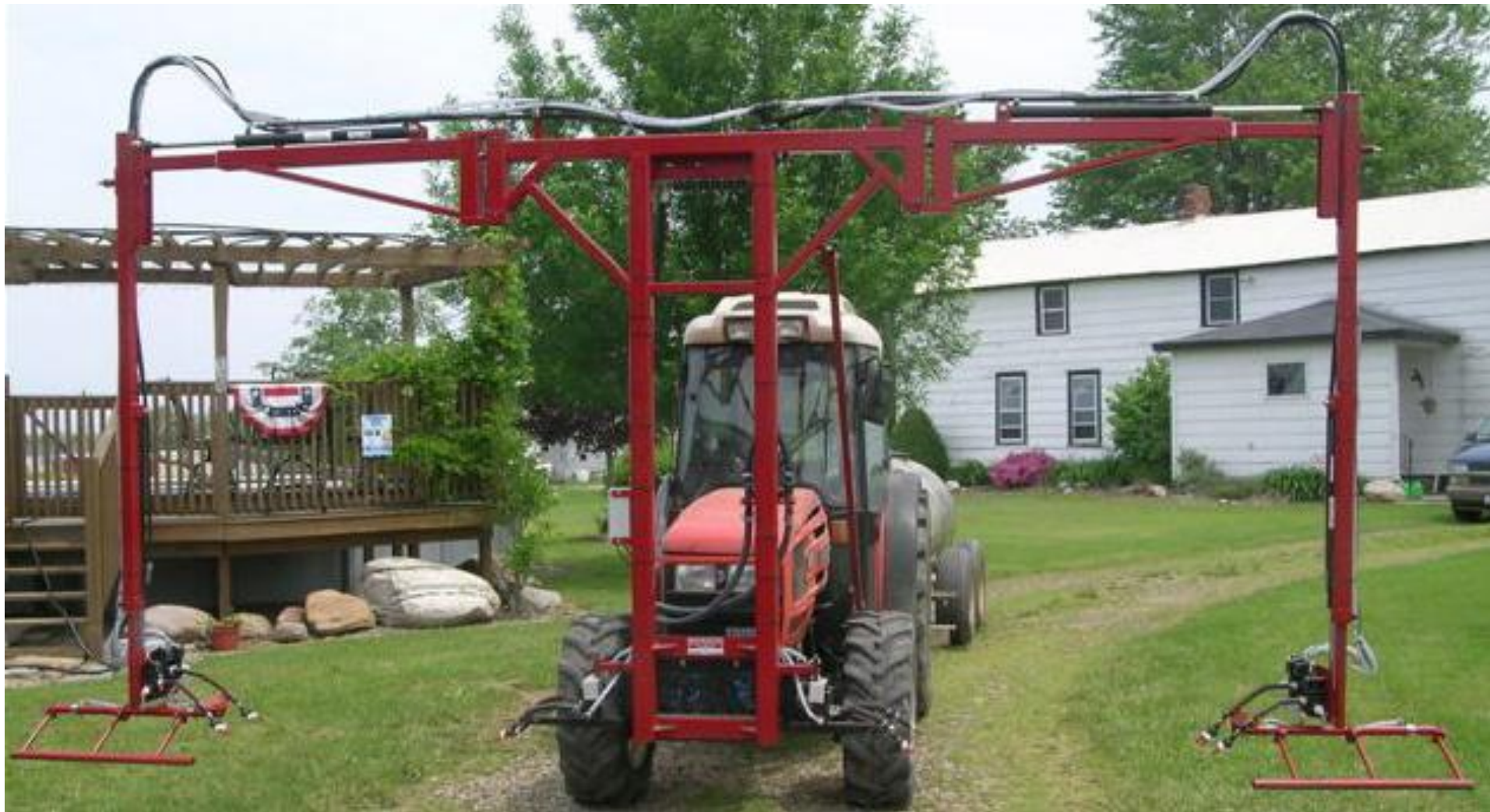
Custom Built Two-Row Vineyard Herbicide Sprayer Capable of Spraying Two Full Rows (Under-Vine and Row Centers) Simultaneously
